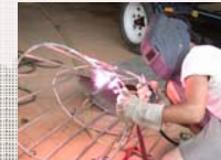
Welding repair of harvest basket
