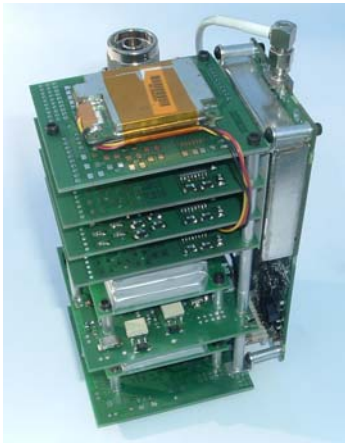
Fig. 7: Main Command Pod electronics with Zigbee wireless to Experiment Pods, 110 kbit spread Spectrum telemetry and command link. Also includes GPS, Battery, data storage, processors, and
