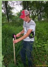
Figure 2 – Placing lathe to outline the boundaries of a wetland on the banks of the Fox River.
